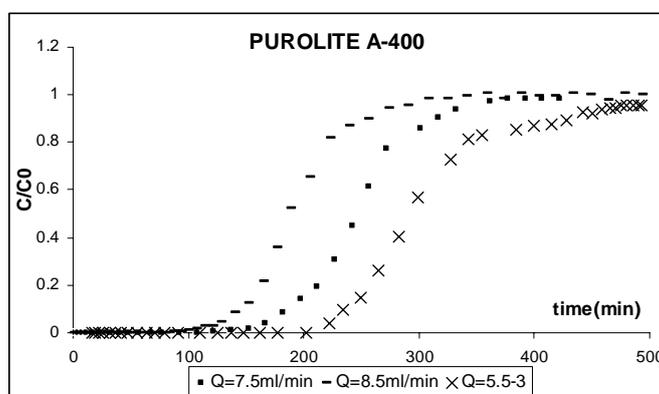
Fig. 1. Effect of flow rates on breakthrough curves by PUROLITE A-400 at 600ppm initial solution concentration of salicylic acid
