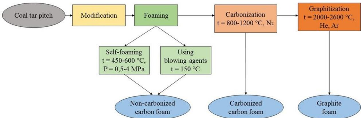
Fig.2. Scheme of carbon foams production
