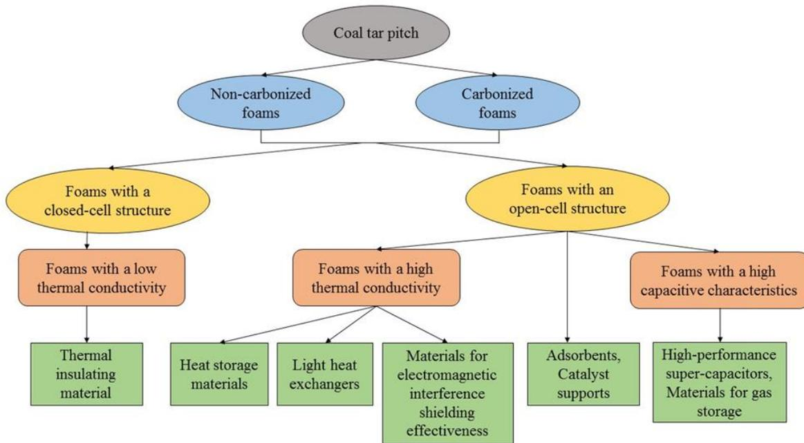
Fig.1. Carbon foams based on coal tar pitch
