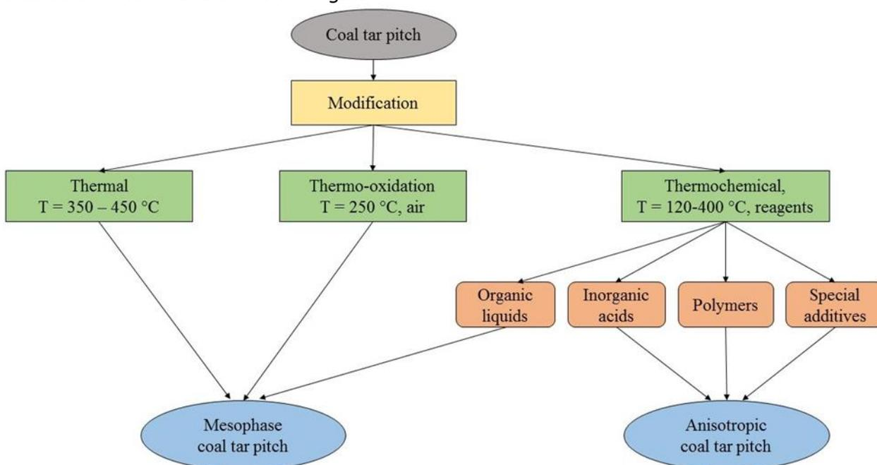
Fig.3. Scheme of coal tar pitch modification methods to obtain carbon foams
