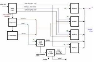
Figure 1 Simplified processing scheme of the Lukoil Neftochim Bourgas Refinery
