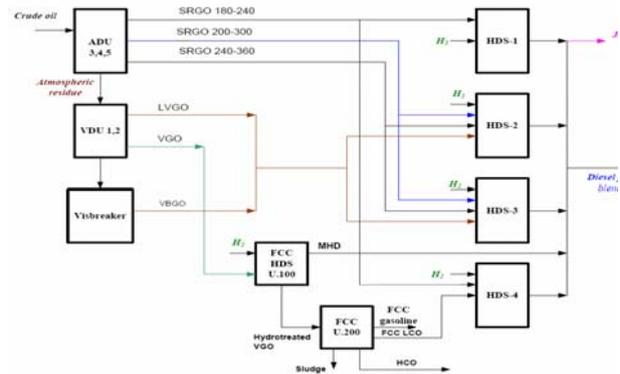
Figure 2. Simplified technological scheme for production of automotive diesel in the LNB refinery
