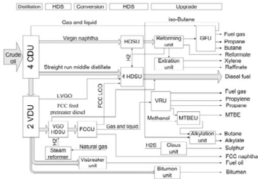
Figure 1 Simplified processing scheme of the Lukoil Neftochim Bourgas Refinery
