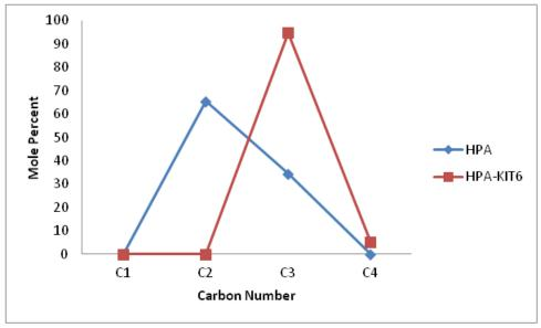
Fig. 4 Carbon number distribution of gaseous product from catalytic degradation of LDPE
