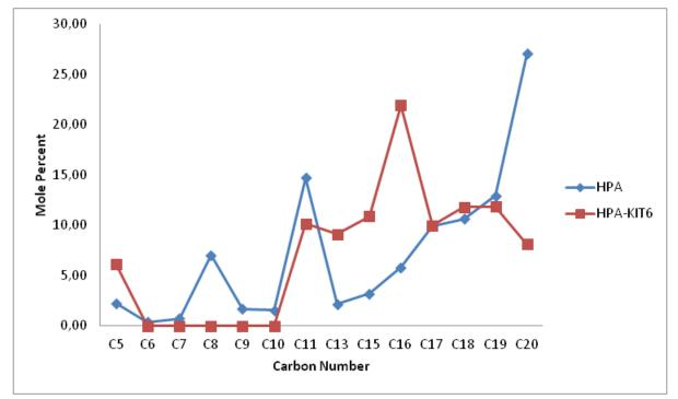
Fig. 5 Carbon number distribution of liquid product from catalytic degradation of LDPE using HPA and HPA-KIT-6.
