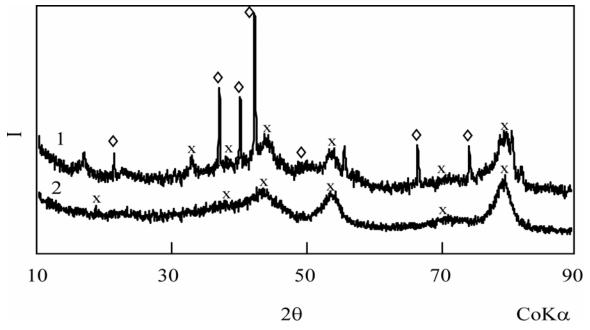
**Fig. 4.** Comparison of the catalysts diffractions before (1) and after (2) the process of methyl chloride hydrolysis was conducted.  $\Diamond - ZnO$ ,  $\times - Al_2O_3$ , I - the number of counting.
