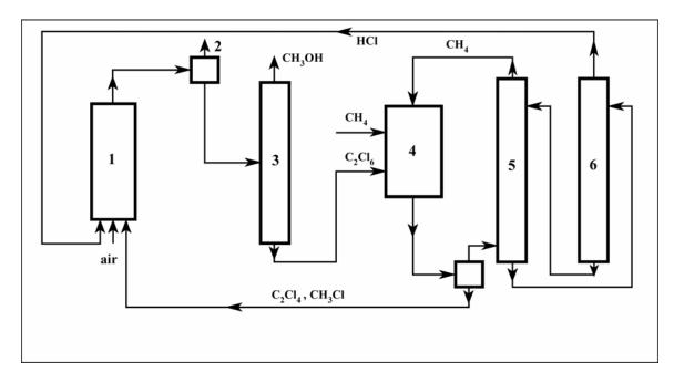
**Fig. 1.** The diagram of the production of methyl alcohol from methane while the process of perchloroethylene oxychlorination is applied. 1 – Catalytic reactor, 2 – Vent, 3 – Distillation column, 4 – Thermal reactor, 5 – Absorber, 6 – Stripper.
