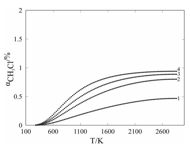
Fig. 2. The dependency of the conversion of methyl chloride into methanol on the temperature of the conducted process.  $1 - CH_3CI : H_2O = 1 : 1; 2 - CH_3CI : H_2O = 1 : 5; 3 - CH_3CI : H_2O = 1 : 10; 4 - CH_3CI : H_2O = 1 : 20.$
