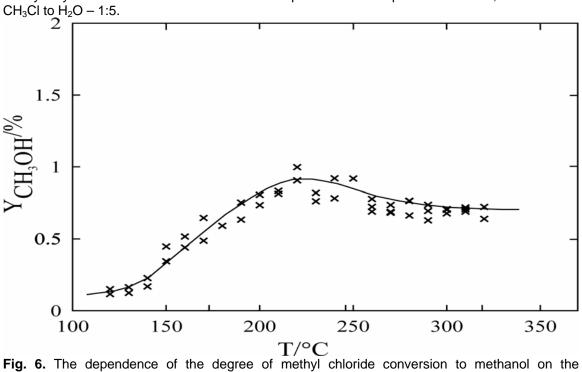
**Fig. 6.** The dependence of the degree of methyl chloride conversion to methanol on the temperature of the conducted hydrolysis. The conditions of the process being run: the flow ratio of  $CH_3CI$  to  $H_2O - 1.5$ .
