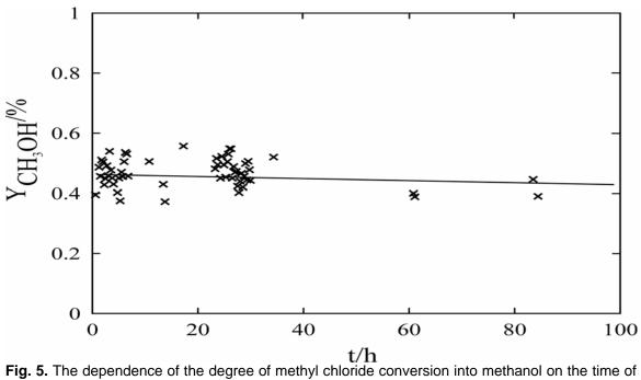
**Fig. 5.** The dependence of the degree of methyl chloride conversion into methanol on the time of the hydrolysis. The conditions of the conducted process: the temperature –  $300^{\circ}$ C; the flow ratio CH<sub>3</sub>Cl to H<sub>2</sub>O – 1:5.
