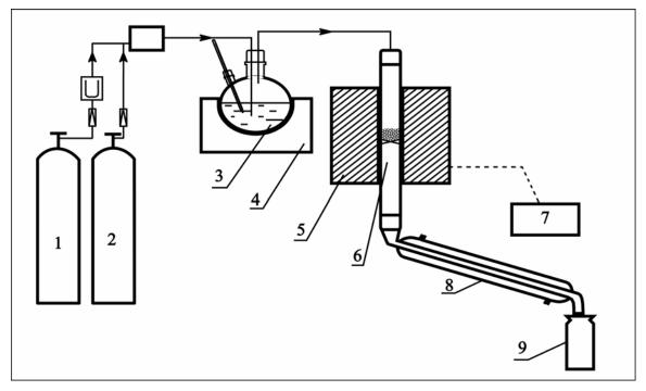
**Fig. 3.** The diagram of the apparatus used for conducting the reaction of methyl chloride hydrolysis.  $1 - CH_3CI$ ,  $2 - N_2$ , 3 - A flask with  $H_2O$ , 4 - A heating jacket, 5 - Furnace, 6 - Reactor, 7 - The temperature control system, <math>8 - Water cooler, 9 - Products receiver.
