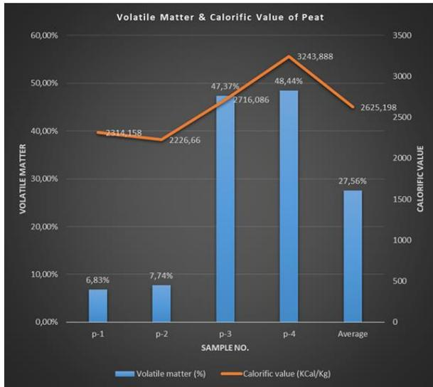
Figure 3. The combined graph of volatile matter and calorific value with their percentage of the peat samples
