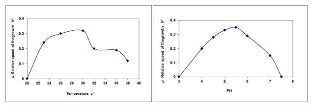
Fig 1 The effect of temperature on the relative speed for the growth of the mixed culture
