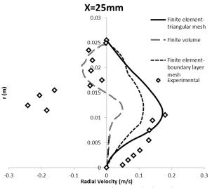
Fig. 11. Variation in the radial velocity at X=25mm
