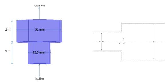
Fig. 1. The computational domain and Fig. 2. Schematic diagram of experimental geometry specifications
