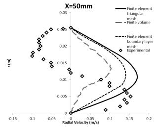
Fig. 9. Variation in the axial velocity at X=50mm
