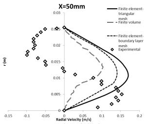
Fig. 13. Variation in the radial velocity at X=50mm
