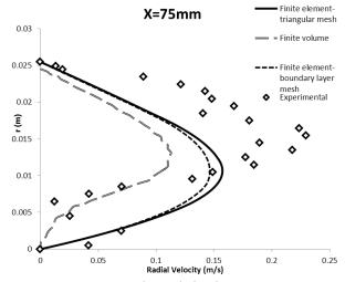
Fig. 13. Variation in the radial velocity at X=75mm
