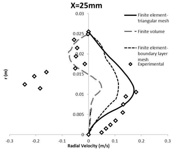
Fig. 11. Variation in the radial velocity at X=25mm
