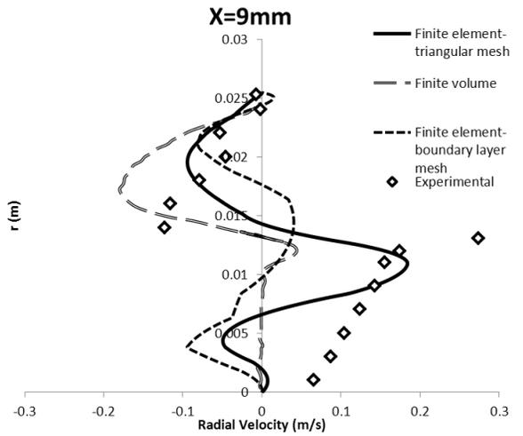
Fig. 10. Variation in the radial velocity at X=9mm
