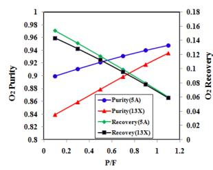
Fig. 6 Oxygen purity and recovery as a function of P/F
