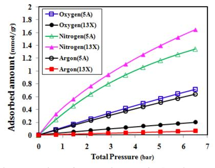
Figure 3 Adsorption isotherm of O<sub>2</sub>, N<sub>2</sub> and Ar on zeolite 5A and 13X at 293.15K.
