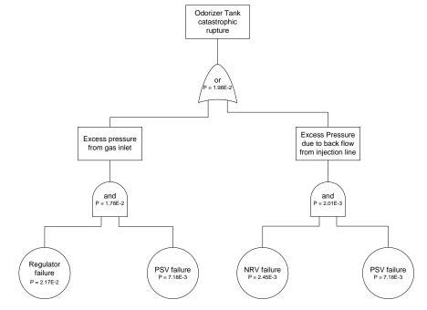
Figure 4. FTA analysis for failure frequency assessment
