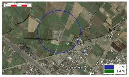
Figure 3. Flash fire maximum effect zone in windy weather
