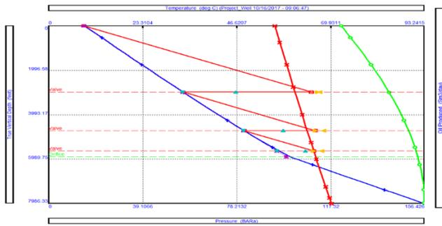
Figure 3. Case 2, Gas lift Design Plot
