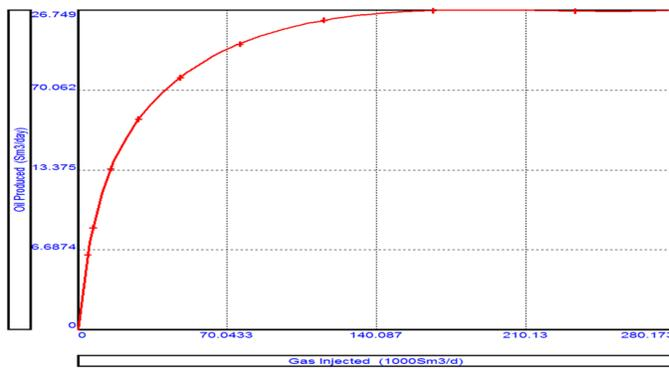
Figure 2. Case 1, Gas lift performance curve
