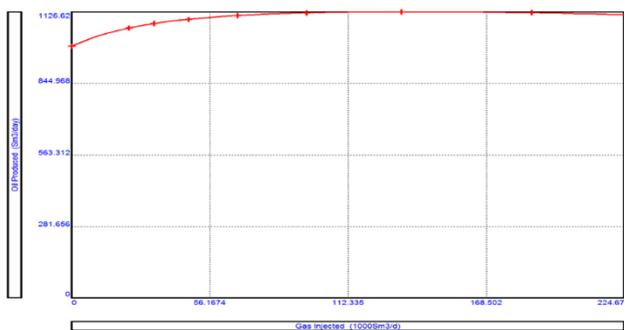
Figure 4. Case 3, Gas lift performance curve
