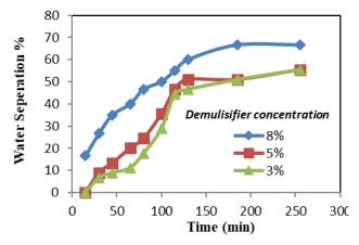
Fig. 4 Effect of the demulsifier concentration at constant temperature 70°C, water content 30% and salt content 3%
