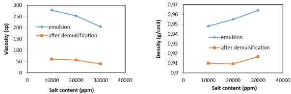
Fig. 10 Effect of salt content on viscosity at water content 30%, demulisifier concentration 8% and temperature  $70^{\circ}C$
