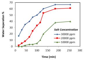
Fig. 6. Effect of salt content at constant demulsifier concentration 8%, temperature70°C and water content 30%
