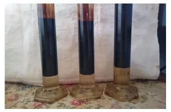
Fig. 1. Crude oil after separation process
