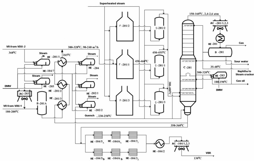
Legend: C- Column; F – Furnace; D – Drum; S –Soaker; AC – Air Cooler; HE – Heat exchanger
