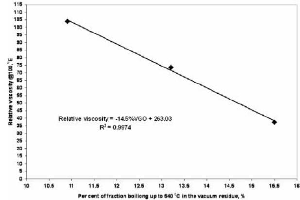
Figure 3 Relationship between vacuum residue relative viscosity and content of fraction distilled up to  $540^{\circ}\text{C}$  in it
