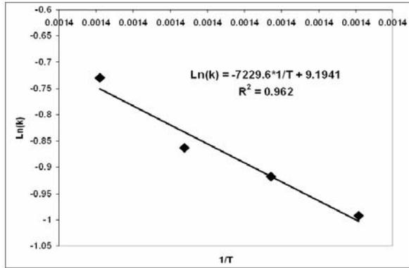
Figure 2 Arrhenius form plot for the temperature dependence of kinetic constant k
