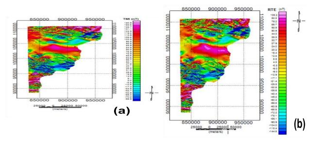
Fig. 2a and b. Total magnetic intensity and residual maps of the study area respectively
