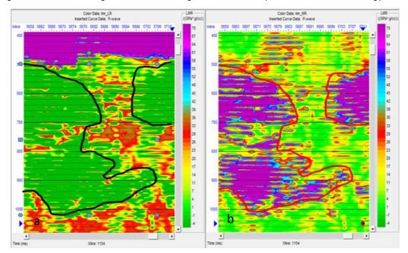
Fig.7. Lambda-Mu-Rho (LMR) inversion (a) Inverted LambdahRho volume (b) Inverted MuRho volume
