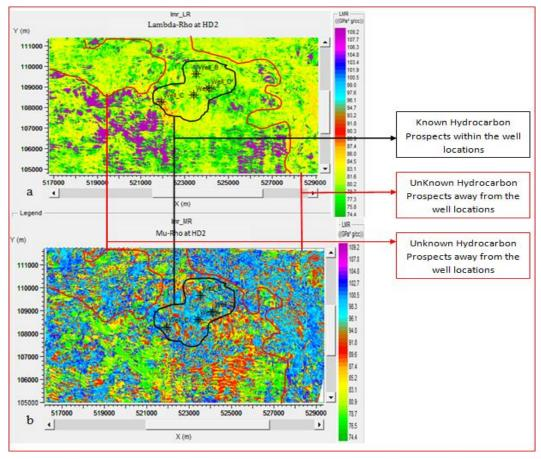
Fig. 8. HD2 reservoir data slices of the inverted (a) LambdahRho (b) MuRho
