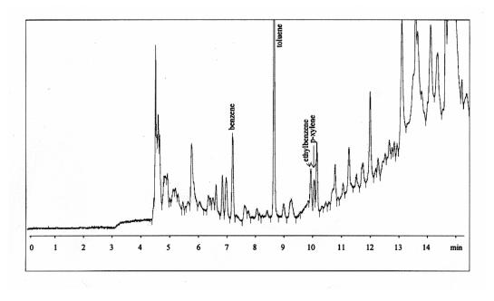
Figure 3. Chromatogram from the analysis of 200 ml air sample from town crossroad.
