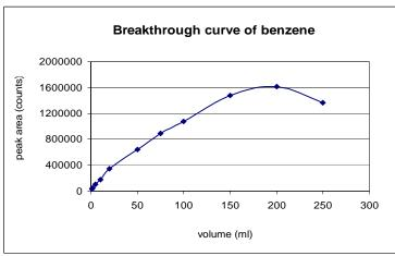
Figure 2. Model gaseous sample volume dependence of chromatographic peak area of benzene at level of 220  $\mu$ g/l.
