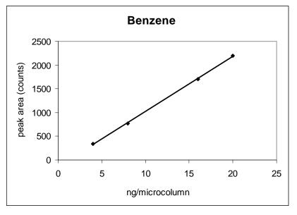
Figure 1. Calibration line for benzene.
