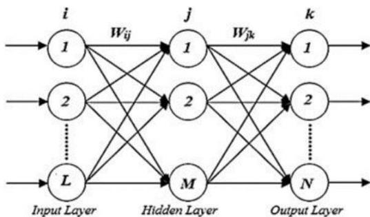
Fig. 1 Structure of an Artificial Neural Network
