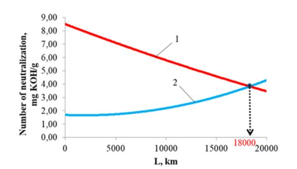
Figure 14. Dependence of the neutralization number on L for oil API SG/CD 15W-40: 1 – TBN; 2 – TAN.
