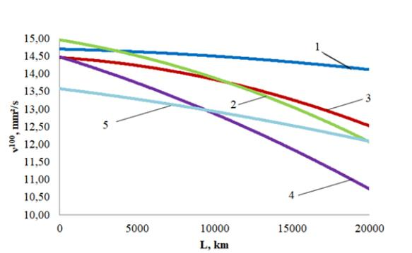
Figure 4. Dependence of  $v^{100}$  on L for mineral oils: 1 – Shell Rimula r4 x 15W-40; 2 – Fuchs Titan Truck Plus 15W-40; 3 – GT Super Diesel 15W-40; 4 – Titan UHPD 15W-40; 5 – API SG/CD 15W-40
