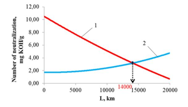
Figure 11. Dependence of the neutralization number on L for oil Shell Rimula r4 x 15W-40: 1 – TBN; 2 – TAN.
