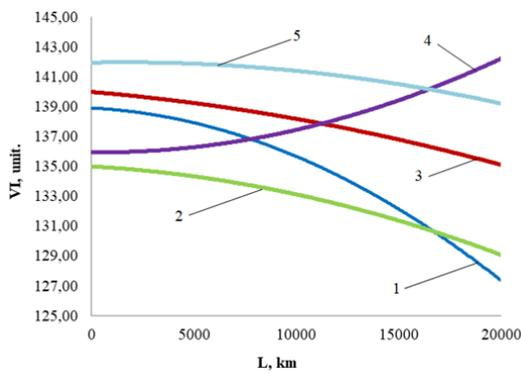
Figure 3. Dependence of VI on L for mineral oils: 1 – Shell Rimula r4 x 15W-40; 2 – Fuchs Titan Truck Plus 15W-40; 3 – GT Super Diesel 15W-40; 4 – Titan UHPD 15W-40; 5 – API SG/CD 15W-40
