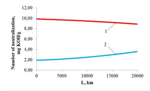
Figure 13. Dependence of the neutralization number on L for oil Fuchs Titan Truck Plus 15W-40: 1 – TBN; 2 – TAN.
