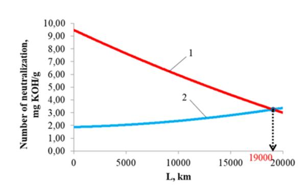
Figure 12. Dependence of the neutralization number on L for oil GT Super Diesel SAE 15W-40: 1 – TBN; 2 – TAN.
