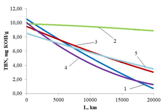
Figure 6. Dependence of TBN on L for mineral oils: 1 – Shell Rimula r4 x 15W-40; 2 – Fuchs Titan Truck Plus 15W-40; 3 – GT Super Diesel 15W-40; 4 – Titan UHPD 15W-40; 5 – API SG/CD 15W-40.
