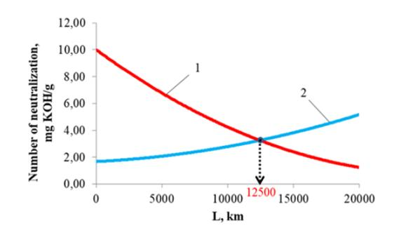
Figure 10. Dependence of the neutralization number on L for oil Titan UHPD 15W-40: 1 – TBN; 2 – TAN.
