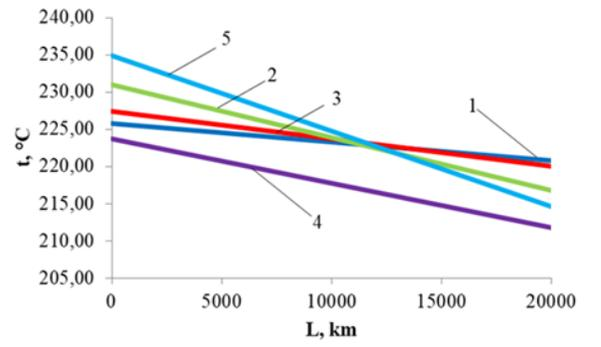
Figure 8. Dependence of  $t$  on  $L$  for mineral oils: 1 – Shell Rimula r4 x 15W-40; 2 – Fuchs Titan Truck Plus 15W-40; 3 – GT Super Diesel 15W-40; 4 – Titan UHPD 15W-40; 5 – API SG/CD 15W-40.
