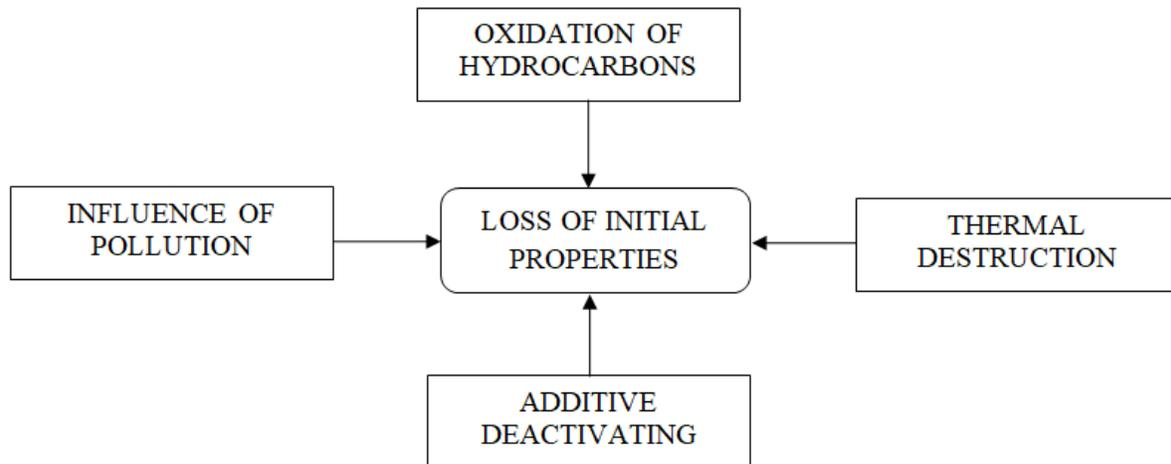
Figure 1. Factors affecting the aging of motor oil in operation.
