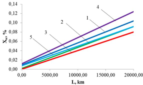
Figure 7. Dependence of  $X_w$  on  $L$  for mineral oils: 1 – Shell Rimula r4 x 15W-40; 2 – Fuchs Titan Truck Plus 15W-40; 3 – GT Super Diesel 15W-40; 4 – Titan UHPD 15W-40; 5 – API SG/CD 15W-40.
