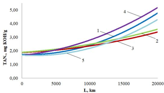
Figure 5. Dependence of TAN on L for mineral oils: 1 – Shell Rimula r4 x 15W-40; 2 – Fuchs Titan Truck Plus 15W-40; 3 – GT Super Diesel 15W-40; 4 – Titan UHPD 15W-40; 5 – API SG/CD 15W-40.
