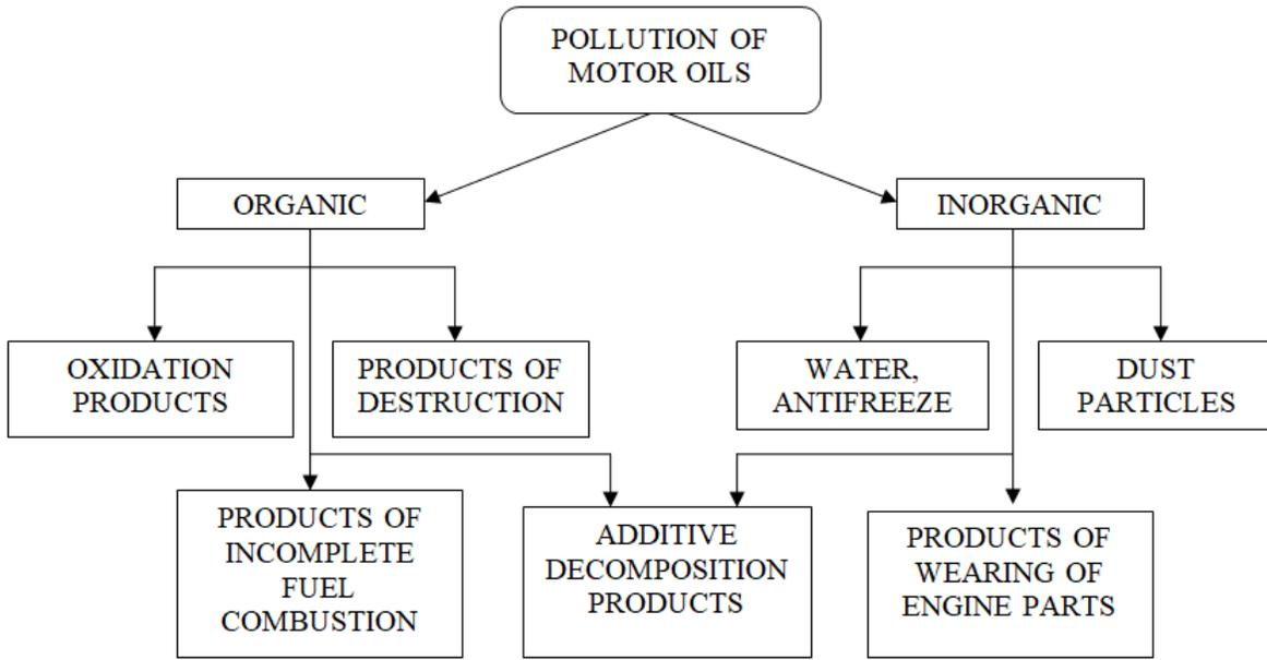
Figure 2. Types of motor oil contamination in operation.
