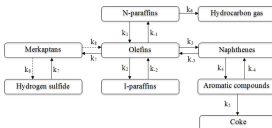
Fig. 2. Formalized scheme of catalytic dewaxing reactions
