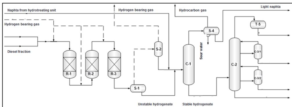
Fig. 1. Industrial diesel fuels catalytic dewaxing unit
