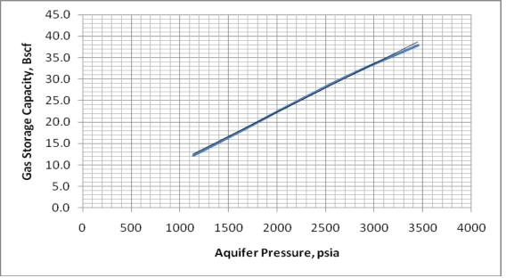
Fig 3.1 A plot of volume of gas to be injected at various pressures for aquifer.
