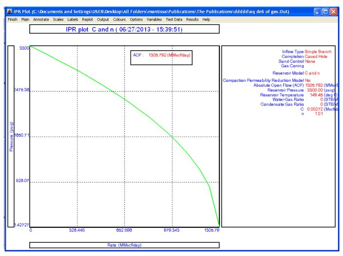
Fig. 3.3 IPR Curve generated with Prosper, a Petroleum Engineering Software, *Source: (Petroleum Experts Limited)*<sup>[14]</sup>
