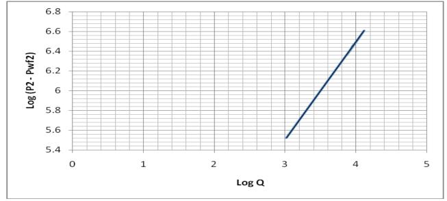
Fig 3.2 Plot of Log  $(P^2 - P_{wf}^2)$  against Log Q
