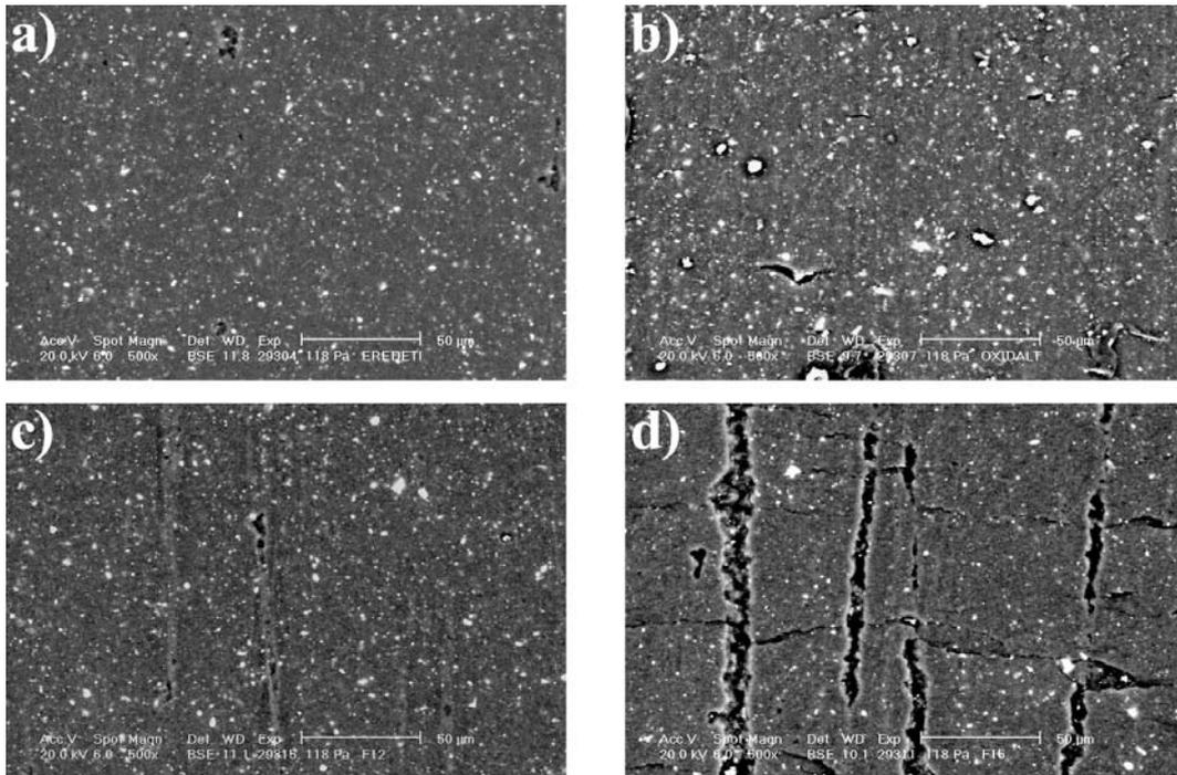
Figure 5 Surfaces of different test-pieces: a) original S3A, b) pre-aged, c) no cracks, d) seriously cracked (ESEM 500x magn.)
