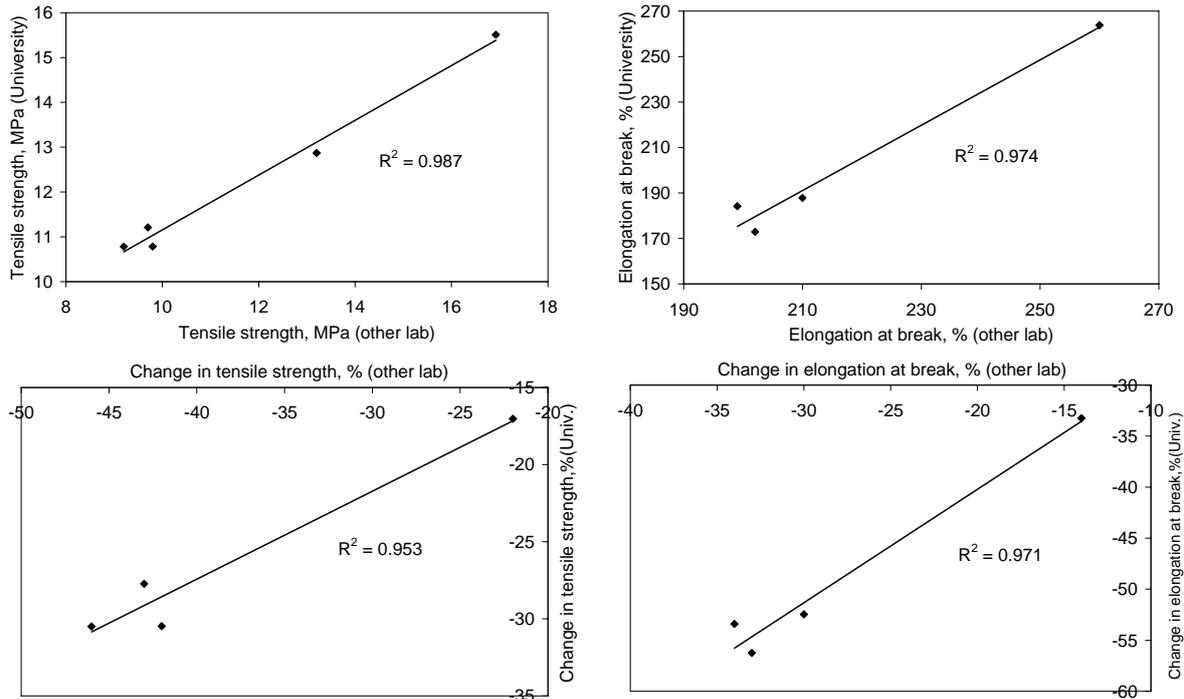
Figure 1 Correlation of the results of the tensile tests (reproducibility)
