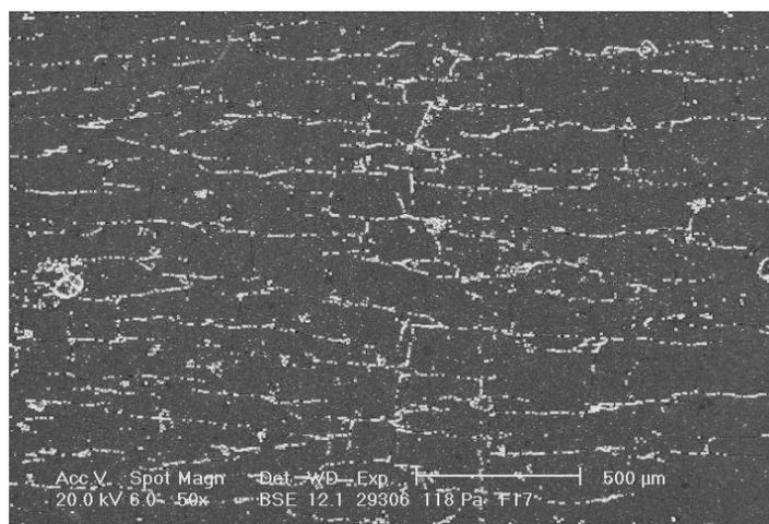
Figure 6 Seriously cracked test-piece of M1 sample (ESEM, 50x magnification), using Adobe Photoshop CS2 the cracks were highlighted by white colour.
