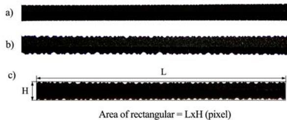
Figure 2 Light cracks (a), serious cracks (b) and the rectangular around the irregular image (c)
