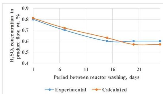
Figure 3. Comparison of the calculated and experimental sulfuric acid yield in February 2020
