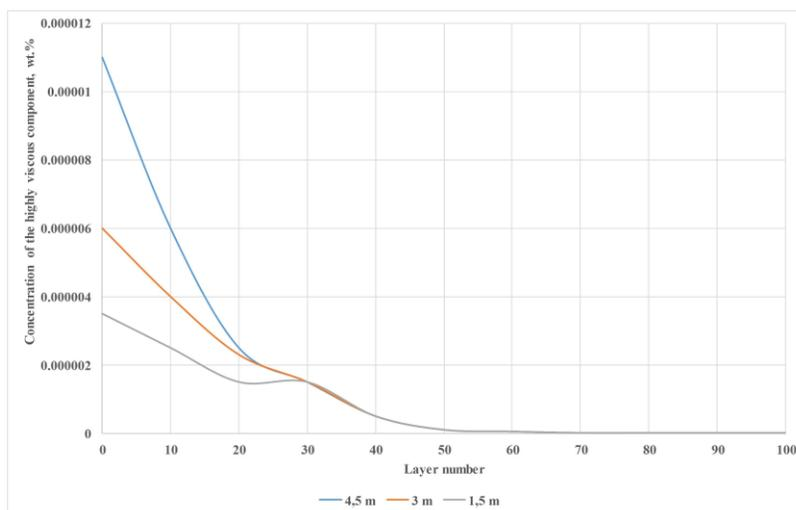
Figure 4. Dynamics of changes in the concentration of a highly viscous component along the vertical and radial axe
