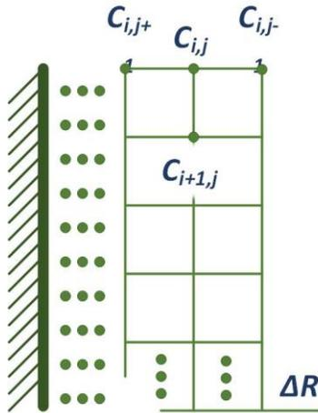
Figure 1. Breaking the liquid film into cells and assigning them indices
