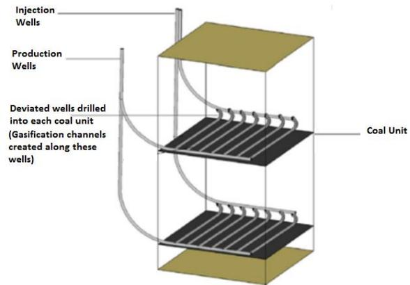
Figure 3. 3D view of well development scheme using CRIP [7]
