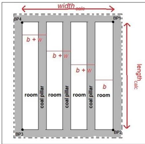
Figure 4. The room and rib pillar configuration general plan view if  $n=3$  (note that the dotted lines represent lateral continuity of coal beyond the area of study). The BP (indicated by black dots) are exactly the same as those identified in Figure 5, when gasification is carried out in the east-west direction
