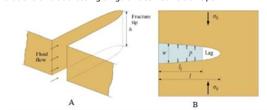
Figure 9. The KGD model: A) the model setup, and B) the plane strain assumption on the horizontal section.
