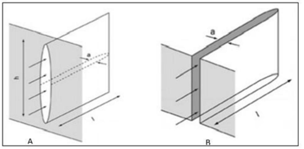
Figure 10. Fracture models. A) PKN model, and B) KGD model [45].
