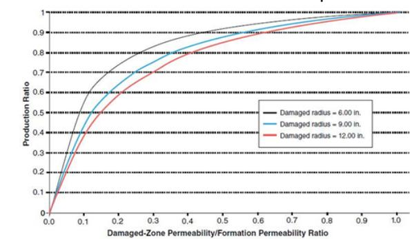
Figure 4. Effect of permeability damage on well productivity.
