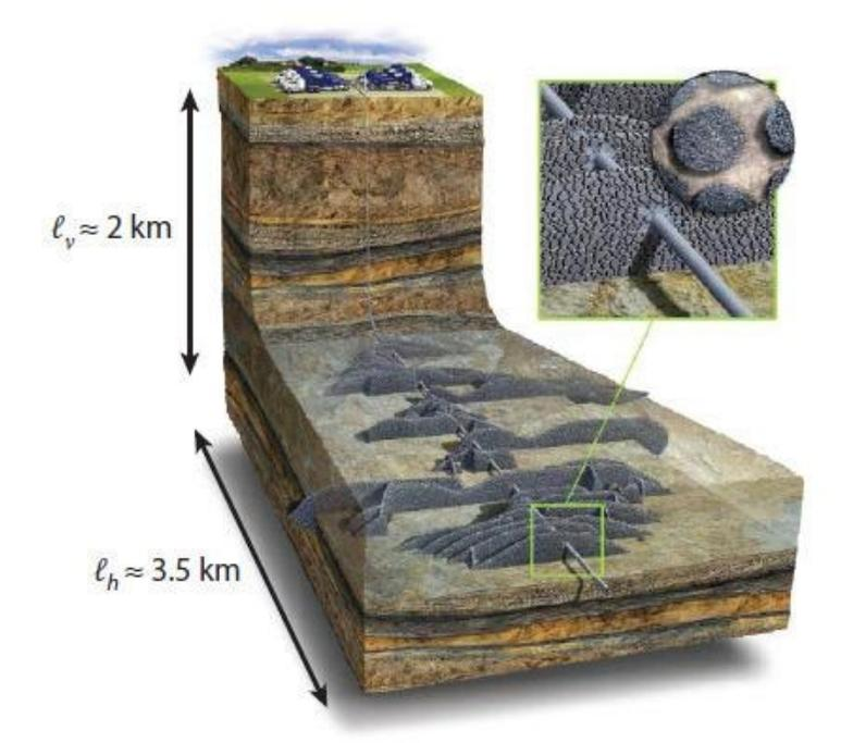
Figure 1. Schematic diagram of a contemporary fracturing job [3].
