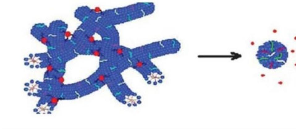
Figure 5. Association of internal breakers (light blue) and nanoparticles (red) with VES micelles.
