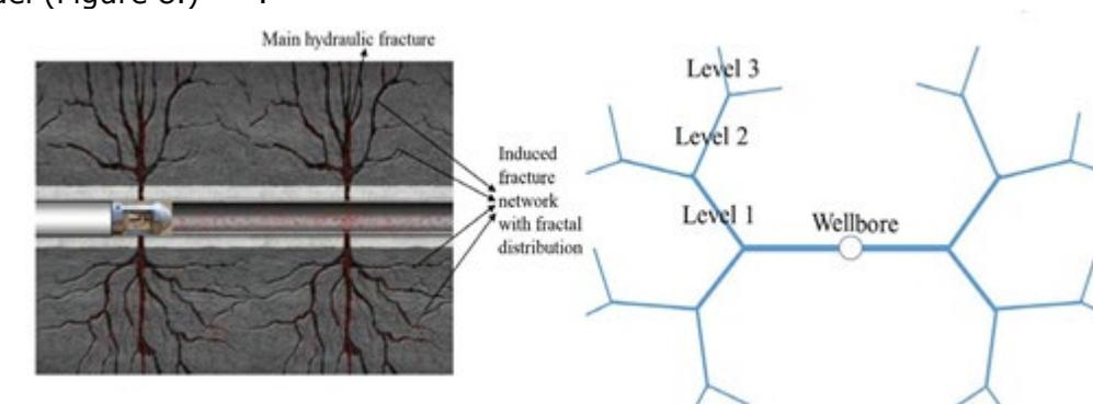
Figure 8. Schematic diagram of fracture morphology of actual and fractal tree [34].
