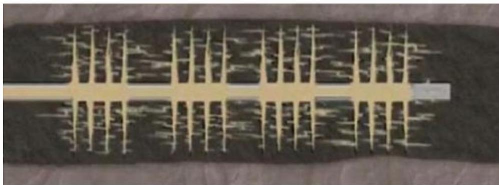
Figure 2. Schematic diagram of hydraulic fracture networks generated by multiple stages in a horizontal well [4].
