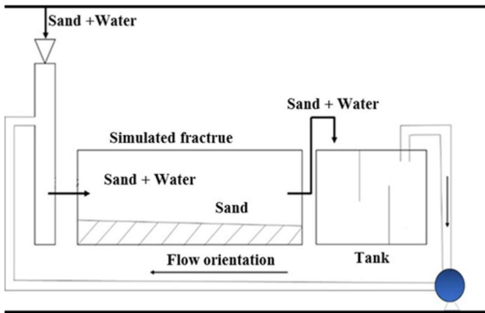
Figure 6. A sand movement equipment [27].
