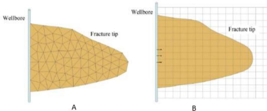
Figure 11. The planar 3D (PL3D) model: A) a moving mesh system, and B) a fixed mesh system.
