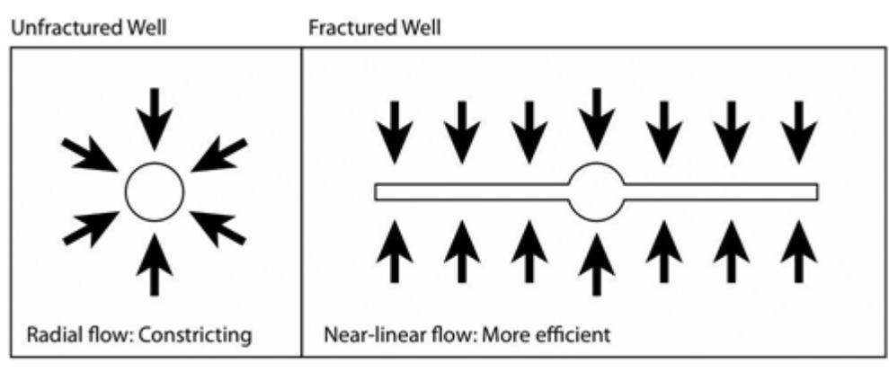
Figure 3. Mechanism of production by hydraulic fracturing.
