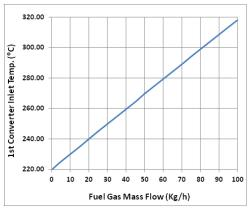
Fig. 4. The changes in temperature of first converter inlet stream vs. mass flow rate of fuel gas inserting into the inline burner
