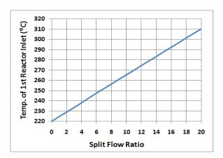
Fig. 3. The changes in temperature of first converter inlet stream vs. hot gas split ratio
