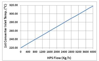
Figure 2. The changes of HPS mass flow vs. the temperature of first converter inlet stream
