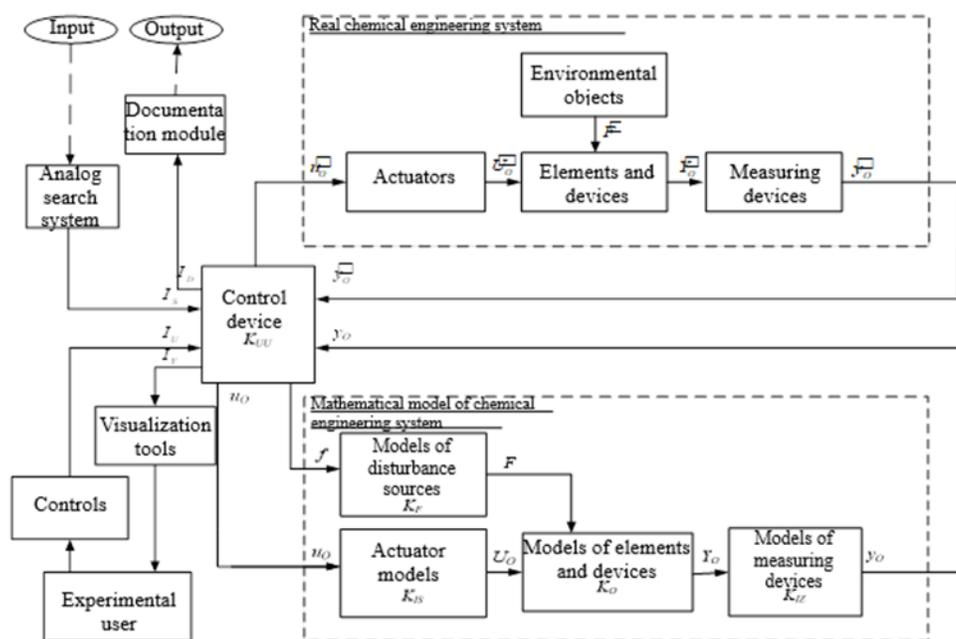
Fig.7. Structure of a computer model of a complex technical controlled system.
