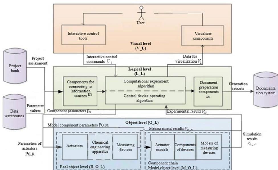
Fig. 6. General structure of a multi-level component chain.
