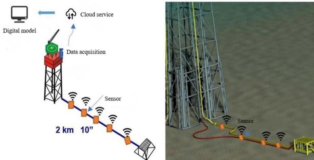
Fig. 5. Location of sensors digital twin data transfer for a subsea pipeline.
