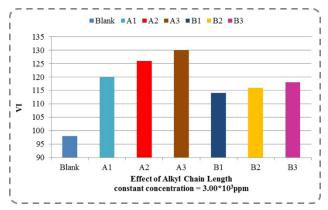
Fig. 1. Effect of alkyl chain length of a- olefin used on VI of lube oil SAE-30 free of Additives
