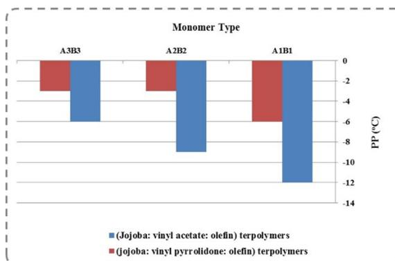
Fig. 3. Effect of Polymer Composition on PP of lube oil SAE-30 Free of Additives
