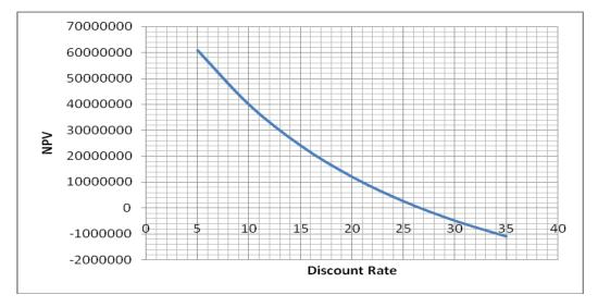
Fig. 2 Plot of NPV against Discount rate, reservoir Z-16T
