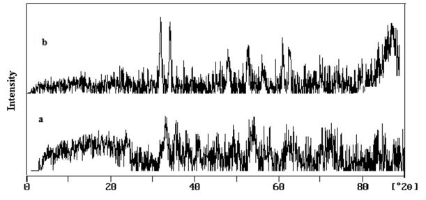
Fig 1. XRD spectra of the fresh catalysts. (a) 100Fe/4Cu (b) 100Fe/4Cu/2Mn
