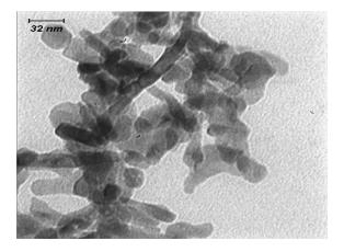
Fig 2. TEM micrograph of the catalyst 100Fe/4Cu/2Mn
