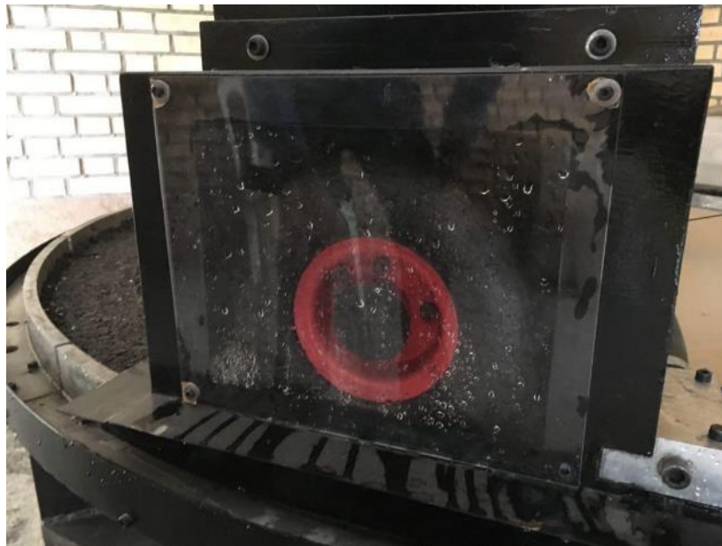
Figure 4. Water transfer between tire and asphalt mixture
