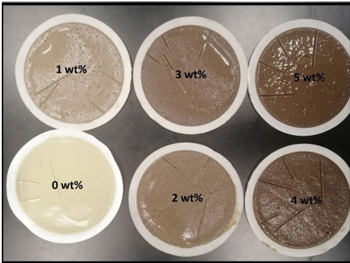
Figure 9. Mud cake with different concentrations of BPP
