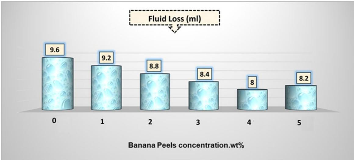
Figure 7. Fluid loss volume at different concentrations of BPP
