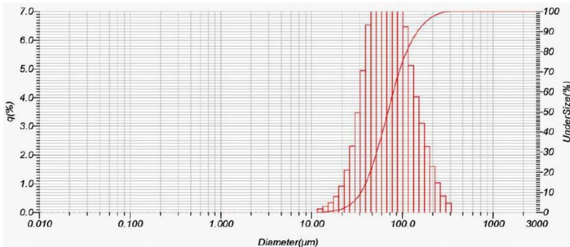
Figure 3. Particle size distribution of BPP
