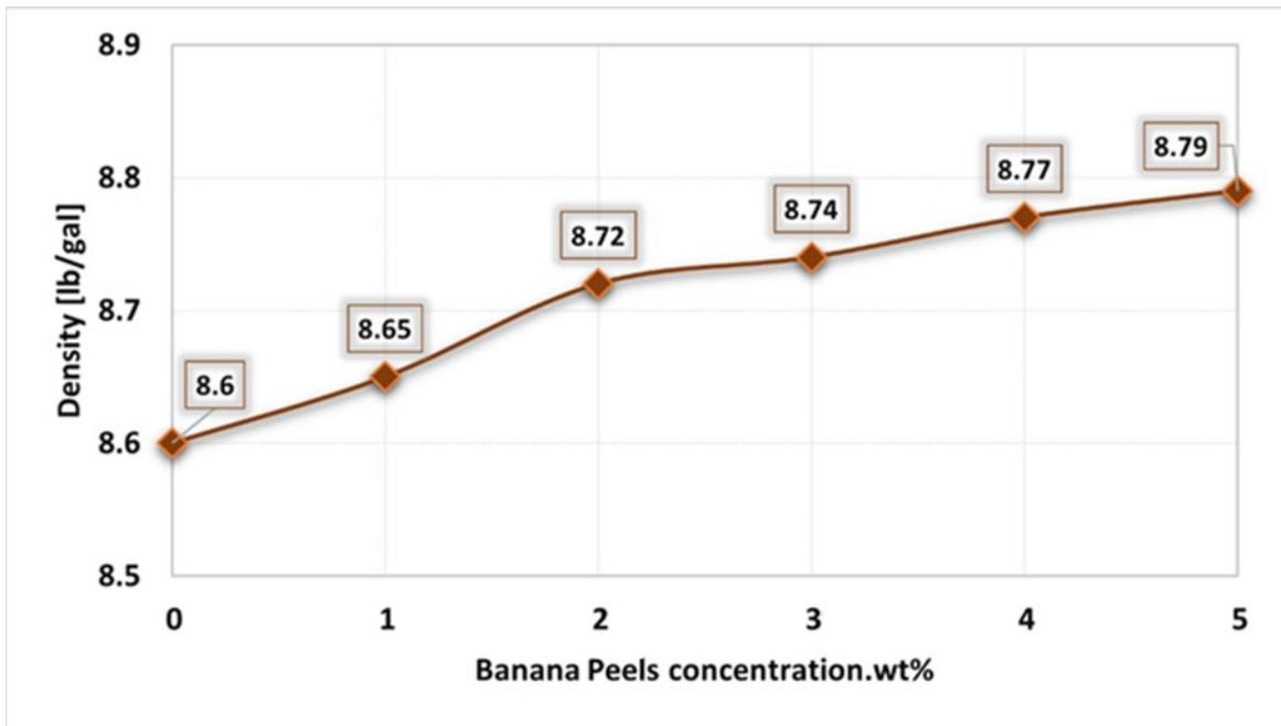
Figure 10. Density of water based mud at different concentration of BPP
