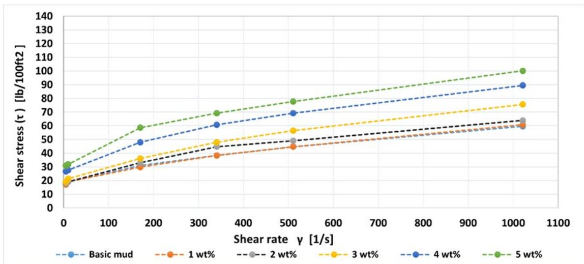
Figure 5. Shear stress via shear rate at different concentrations of BPP
