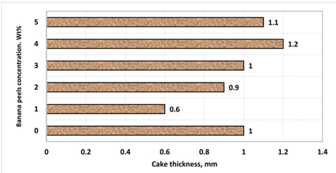
Figure 8. Mud cake thickness at different concentration of BPP
