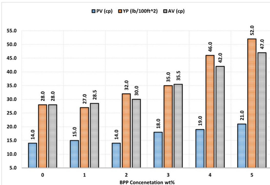
Figure 4. Plastic viscosity, yield point, and apparent viscosity at different concentrations of BPP
