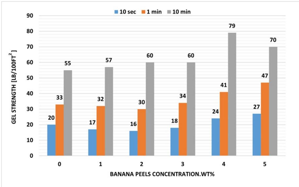
Figure 6. The gel strength of water based mud at different concentrations of BPP
