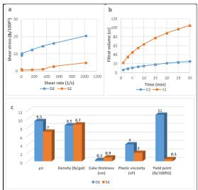
Figure 2. Comparison of rheological properties for S1 and D1 samples, a) Shear rate-shear stress relations b) Time-fluid loss relation, c) pH, density, cake thickness, plastic viscosity, yield point values
