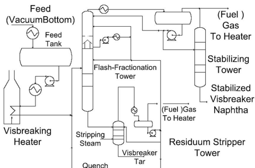
Figure (1): Visbreaking Unit
