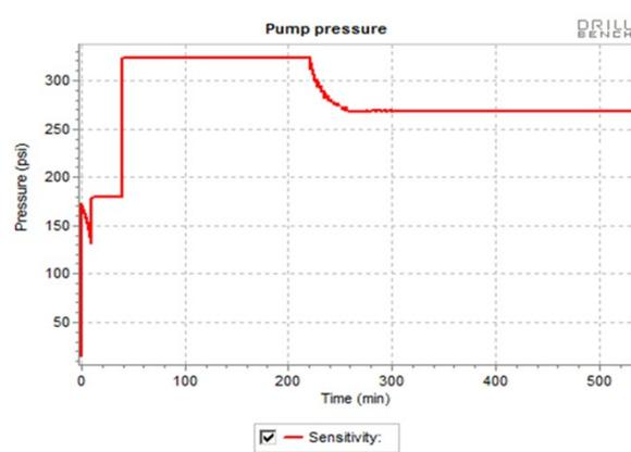
Fig 3. Pump pressure profile using Driller's method
