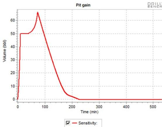
Fig 2. Pit gain profile using Driller's method
