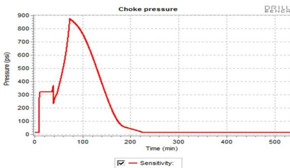
Fig 4. Choke pressure profile using Driller's method
