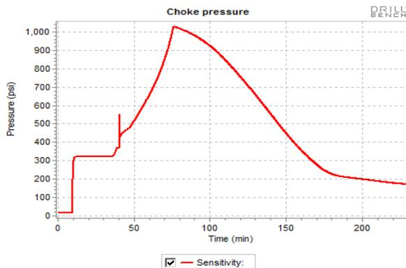
Fig 8. Choke pressure profile using Engineer's method
