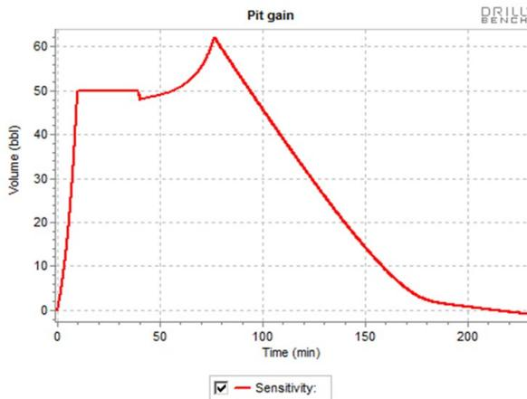
Fig 6. Pit gain profile using Engineer's method
