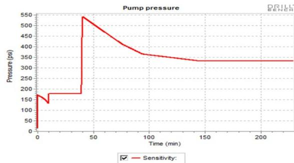
Fig 7. Pump pressure profile using Engineer's method
