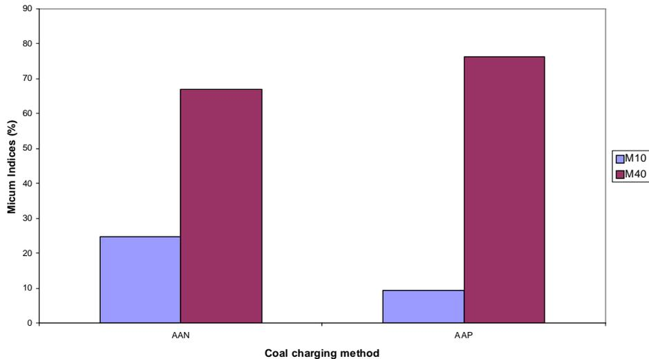
Fig. 1: Effects of coal charging technique on micum indices of resulting coke
