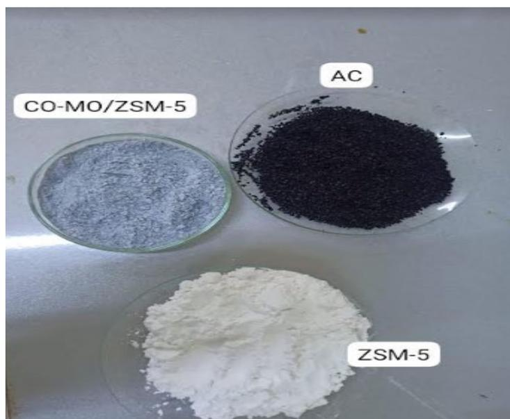
Figure 3. Activated carbon (AC) and the catalyst prepared for the catalytic pyrolysis of waste polypropylene.
