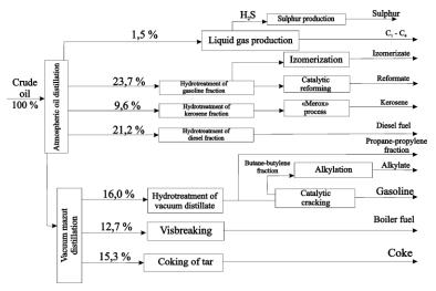
Fig. 1 presents typical structure of oil processing according to the fuel scheme.
