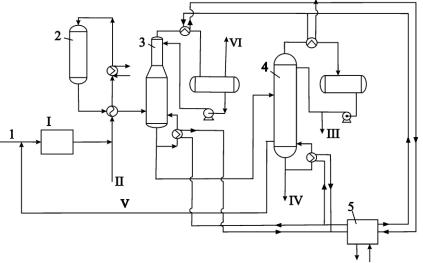
Fig. 4 – Principal scheme of isomerisation unit: 1 – dryer; 2 – reactor of isomerisation; 3 – stabilization column; 4 – deisohexanizer; 5 – ACU; I – raw material, II – hydrogen; III – isomerizate; IV – C7+ fraction; V – recycled material; VI – fuel gas.
