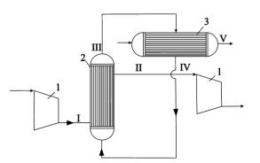
Fig. 5 – Principal scheme of gas cooling with the heat pipe: 1 – compressor; 2 – evaporator of heat pipe; 3 – condenser of heat pipe; I – hot gas; III – cold gas; III – vapour; IV – condensate; V – water
