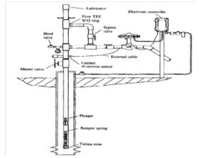
Figure 1. Installation of Plunger lift in a well
