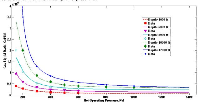
Figure 2. The results of predictive tool for the estimation of minimum gas liquid ration for 2'' plunger lift in comparison with Beeson *et al.*<sup>[3]</sup> data.
