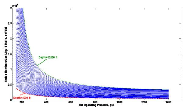
Figure 4. The performance of predictive tool for the estimation of minimum gas liquid ration for 2" plunger lift.
