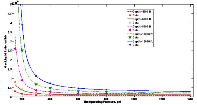
Figure 3. The results of predictive tool for the estimation of minimum gas liquid ration for 2.5" plunger lift in comparison with Beeson *et al.* <sup>[3]</sup> data.
