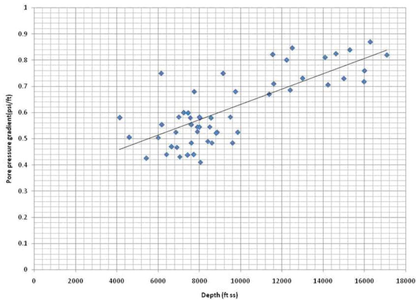
Fig. 11. Pore pressure – depth cross plot showing depth of overpressure occurrence in the study area
