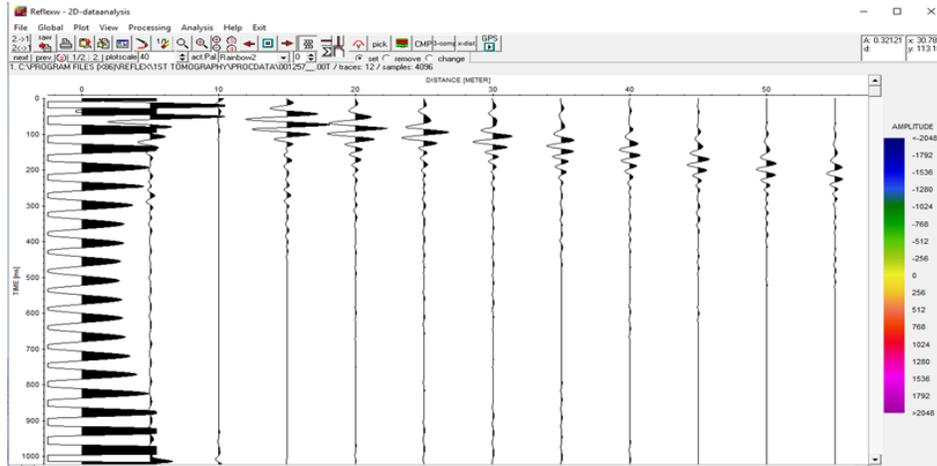
Figure 4. Kicking (traces) after filtering and before gaining
