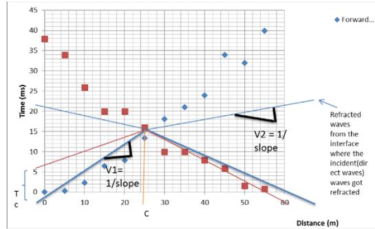
Figure 10. Graph for the 4<sup>th</sup> forward and reverse time
