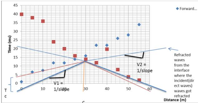
Figure 9 Graph for the 3<sup>rd</sup> forward and reverse time
