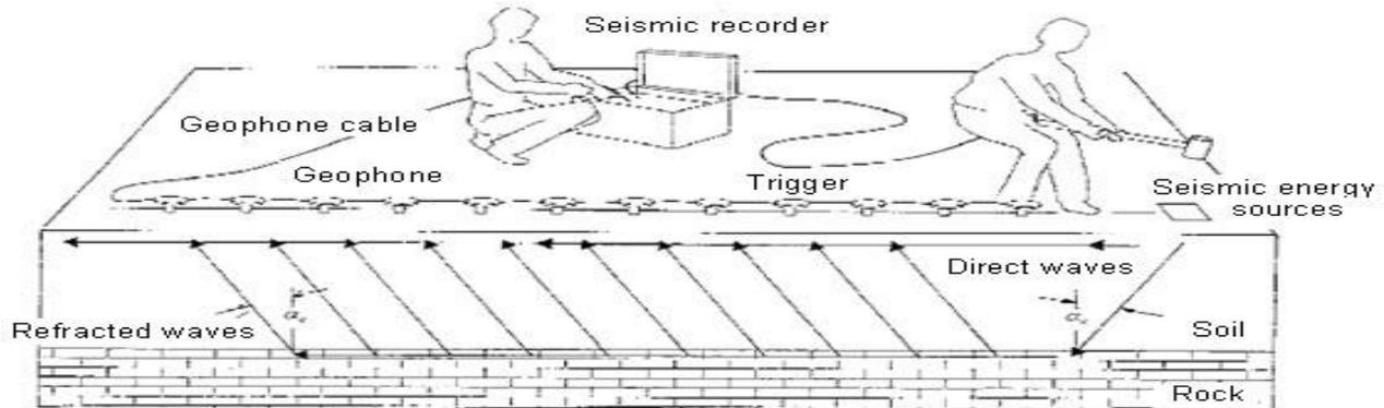
Figure 1: Field layout of seismic refraction [3]
