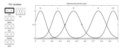
Figure 5. Membership function of input variable gamma ray
