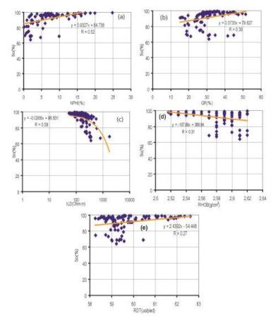
Figure 4. Correlation between inputs log data and oil saturation
