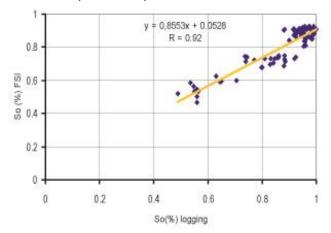
Figure 7. Correlation between oil saturation obtained from logging and that estimated by FSI
