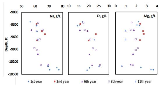
Figure 2. Cation constituents of oilfield produced water at various oil production years and depth
