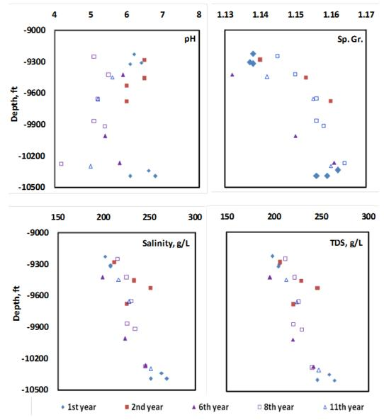
Figure 1. Physical characteristics of oilfield produced water at various oil production years and depths.
