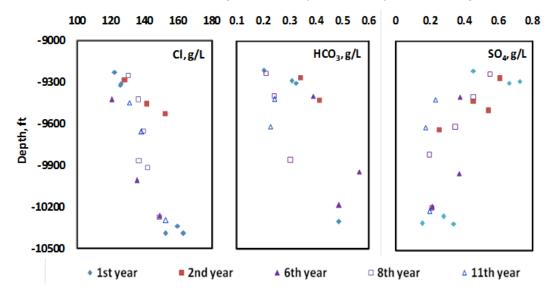
Figure 3. Anion constituents of oilfield produced water at various oil production years and depths.
