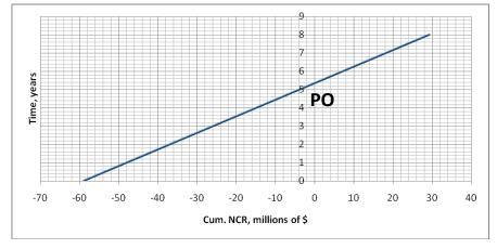
Fig 3.7 Plot of Time in years against Cum NCR in millions of dollars for reservoir Z-16T with water influx
