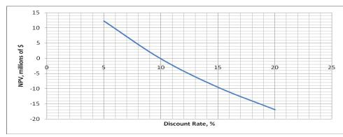
Fig 3.9 Plot of NPV in millions of dollars against Discount Rate in % for reservoir Z-16T with water influx
