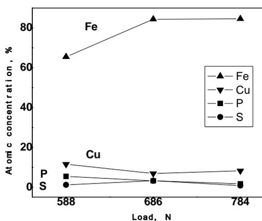
Fig. 4 Atomic concentration (%) of elements on the worn surface with different loads
