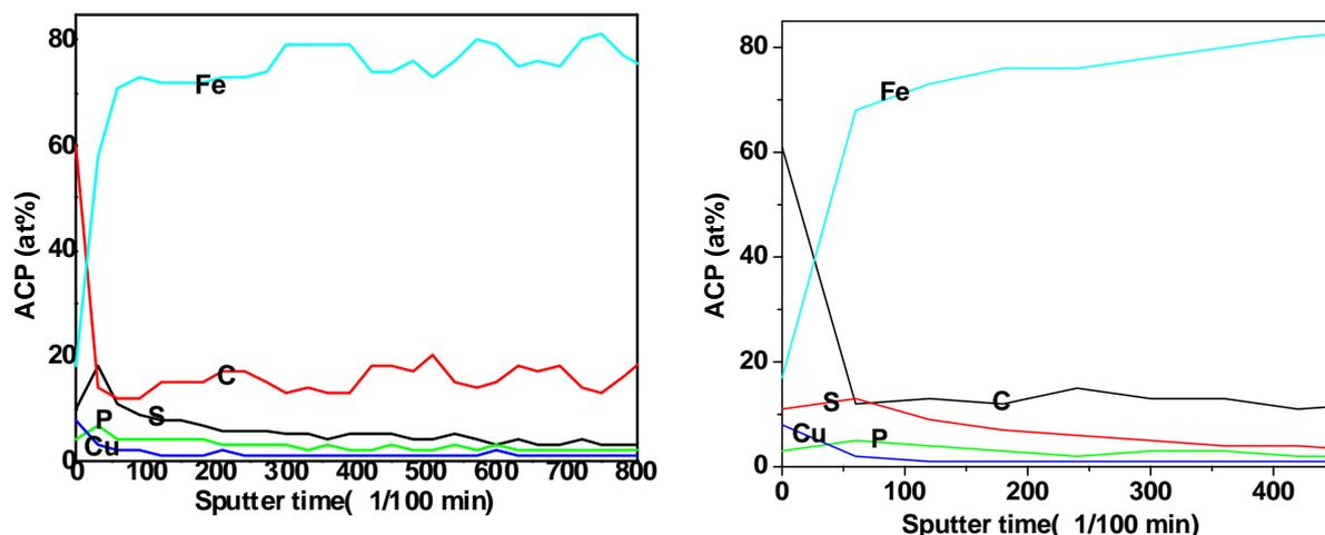
(a) AES depth profile of  $\text{Cu}(\text{DDP})_2$  at a load of 588 N
