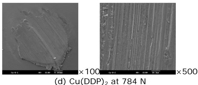
Fig. 3 SEM morphologies of wear scar lubricated with the 500SN,  $\text{Cu}(\text{DDP})_2$  under different load
