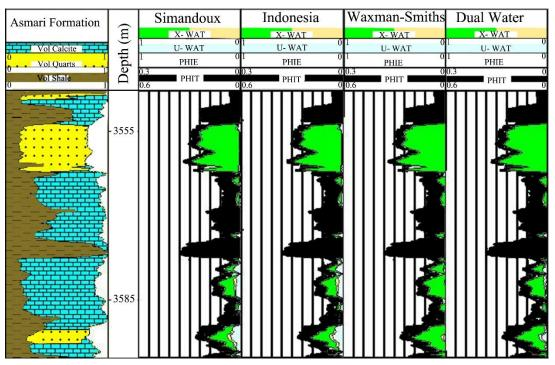
Figure 6. The mixed graph of water saturation models in Kupal oil field, well No.54.
