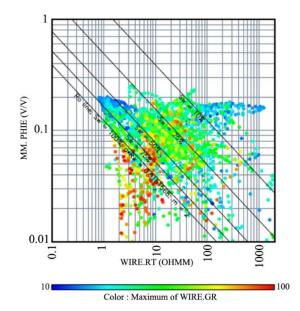
Figure 3. Water saturation (Sw) of Asmari formation for well No.54, based on PHIE to RT  $\,$
