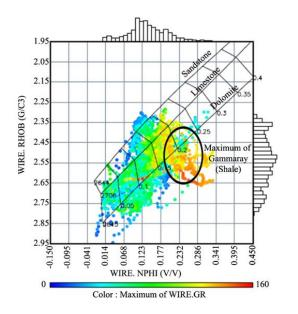
Figure 2. Cross plot of Neutron-Density-GR, Well No.54 in Kupal oil field
