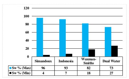
Figure 5. Water saturation percentage in fore models of water saturation
